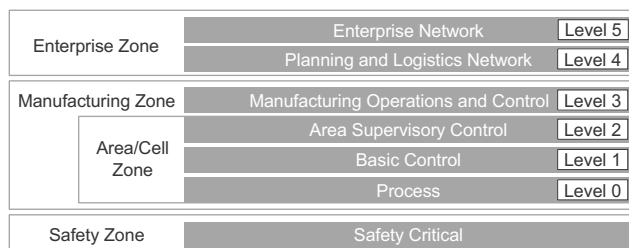
Fig. 3. Purdue Model of Control Hierarchy.
